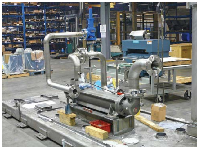
Figure 3. Reduced footprint. The fuel oil system used less than 15 ft of stainless steel piping—a significant achievement providing reduced footprint at the utility and lower material cost.
