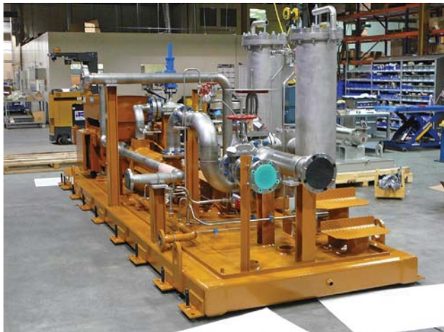
Figure 4. A single package. The fuel oil injection module was an integrated unit containing filtration, fuel injection pump and motor, valves and piping.
