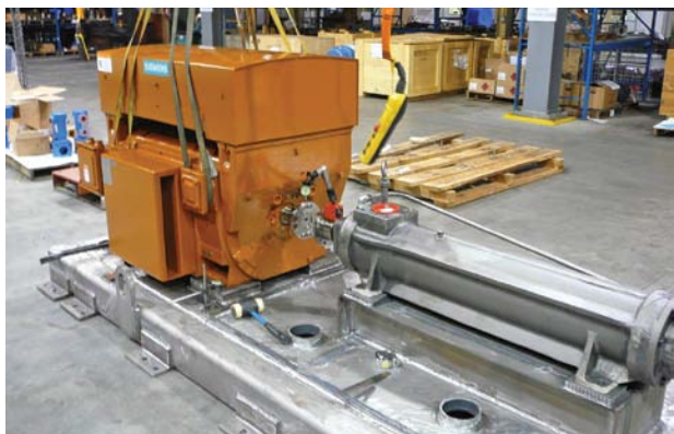
Figure 2. Rotary positive displacement pump. An advanced technology, high pressure, rotary three-screw pump is on the right.
